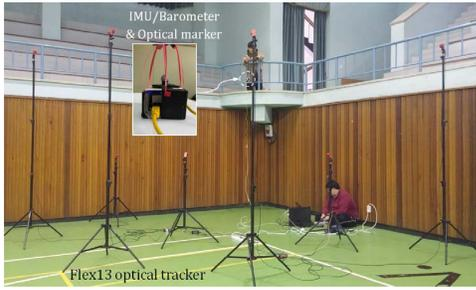
Fig. 3. Test setup with the Fex 13 optical motion capture system in an indoor gym.
